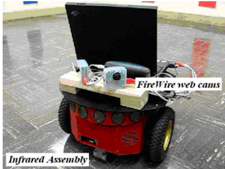
Figure 3.4: Picture of the Pioneer P3-DX robot used in the physical experiments. Two FireWire web cameras are mounted to a wooden base on the front of the robot. An infrared sensor assembly can be seen beneath the front of the robot.
