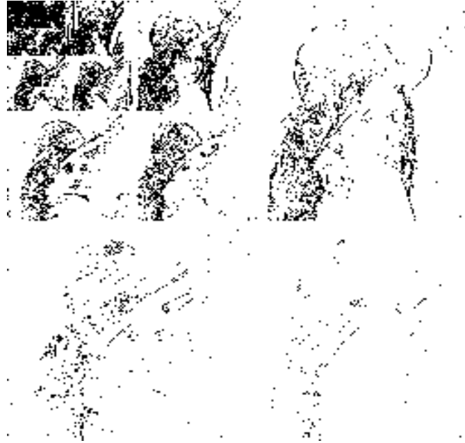
Figure 3.2. The subband pyramid after binary significant map convert
