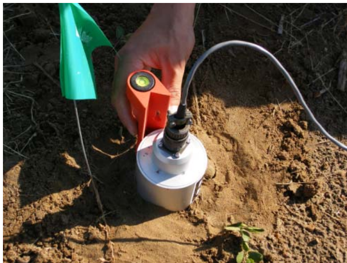
Figure 3.32 Mark Product L-4 high-sensitivity geophone (1 Hz).
