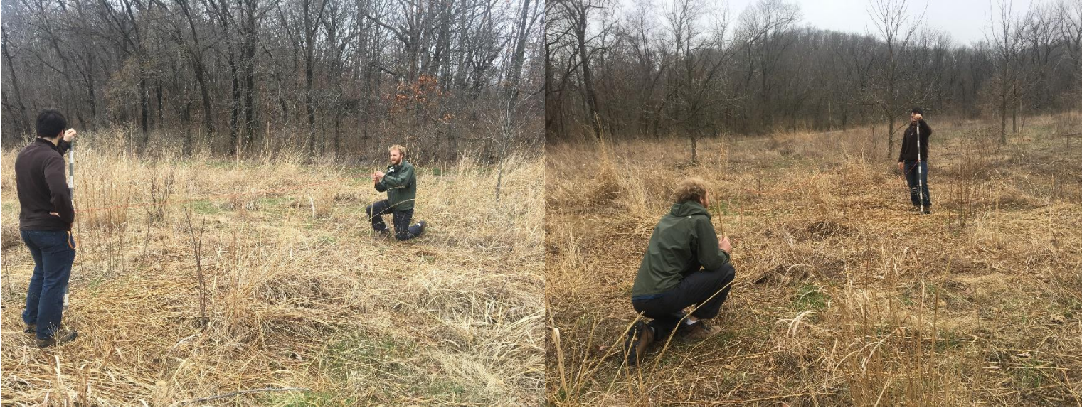
Figure 2.8. Measuring vegetation density with a Robel pole. The observer, positioned 4 meters from the pole at a height of 1 meter, records the lowest visible decameter on the pole.
