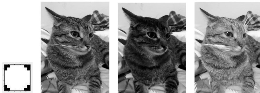
(a) Structuring element (b) original image (c) eroded image (d) dilated image
