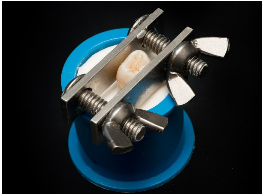
Figure 1. Maxillary third molar mounted in self-curing acrylic resin.
