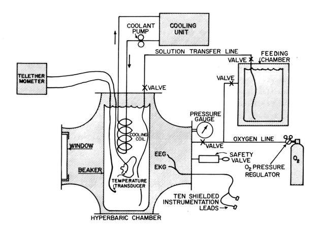
Diagram of Connections for the Hyperbaric Organ Preservation and Reading Chambers.
