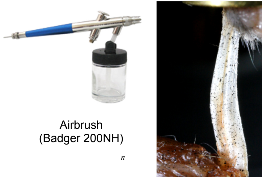
Figure 2-2: Paintbrush and an ulna showing the speckle pattern
