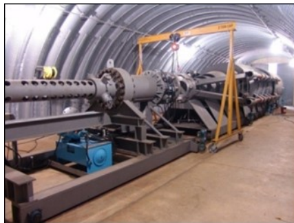
Figure 4.2-1: Blast Load Simulator (Shock tube)
