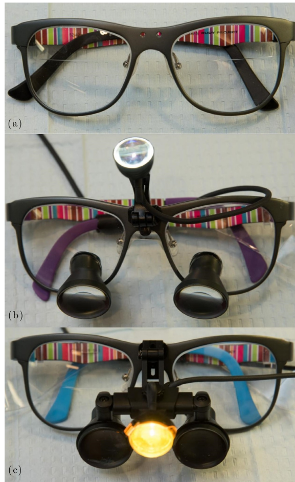
Figure 5.2: (a) Safety lenses with light attachment-no magnification. (Basic eye-wear BL), (b) Through the lens magnification loupes with light attachment. (TTL), (c) Flip Up magnification loupes-with light attachment. (FL)
