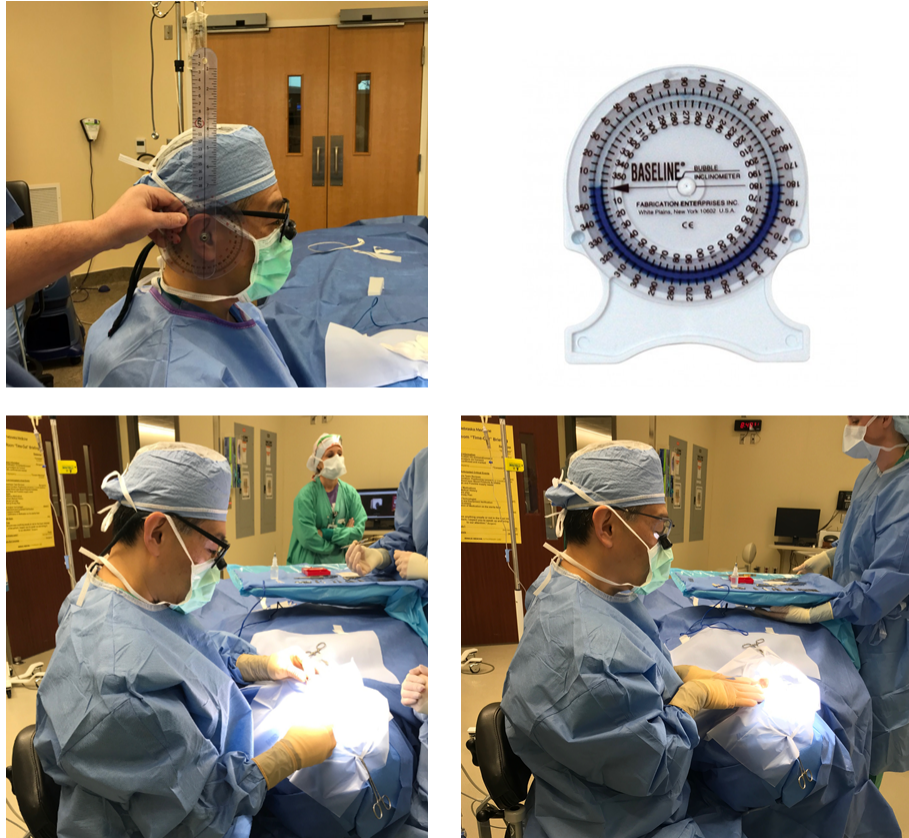
Figure 6.2: Viewing angle determination of the conventional and redesigned loupes in an ophthalmic surgery setting, using a bubble inclinometer
