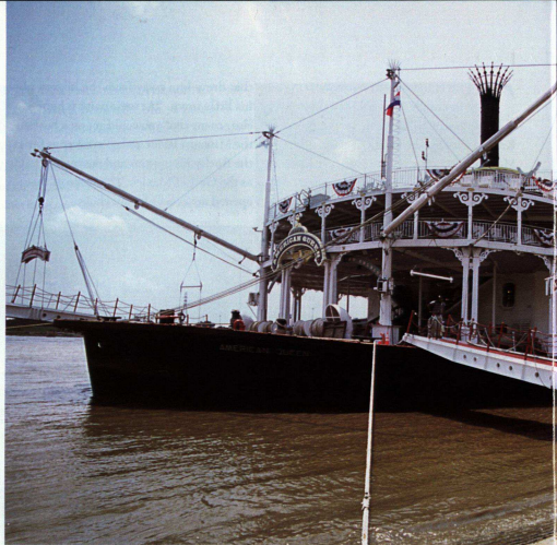
This stack of ornate decks known as the American Queen is in the tradition of boats nicknamed floating wedding cakes. Passengers can walk the balconies for exercise. Two engines totaling 1,500 horsepower turn the 52-ton paddle wheel assembly, right. In wells beneath the painted stars on the deck are a pair of 1,000-horsepower engines, called Z-drives, which turn 5-foot propellers.
