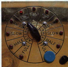
When pilots turn the telegraph's brown dial, bells ring in the engine room, and engineers hustle to execute the speed and directional commands with vintage 1932 engines.
