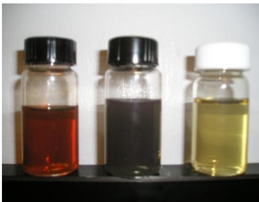
Figure 5. Silver nanoparticles suspensions made from the reduction of silver ion by borohydride in polyvinyl alcohols.
