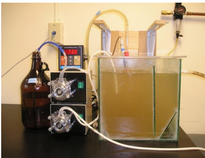
Figure 6. The nitrifying bioreactor used to prepare autotrophic nitrifying bacteria.
