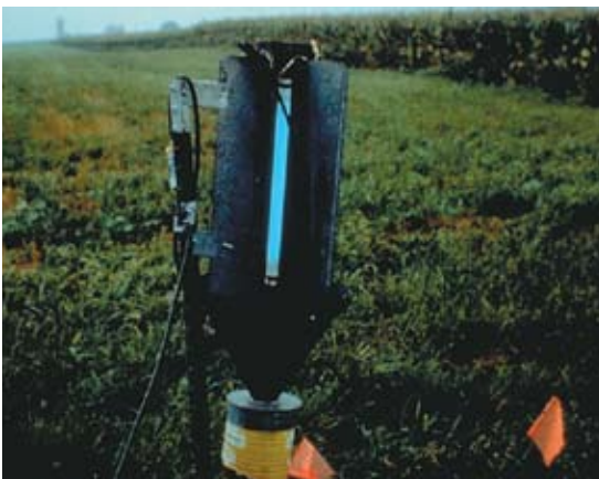
Figure 30. A blacklight insect trap uses a short-wavelength light to attract insects.
