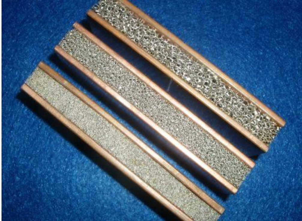
Figure 1.7 Application of Al-foams in high speed trains as a replacement of GFRP
