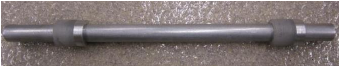
Figure 2.4 Aluminum striker bar with 457.2 mm in length and 12.7 mm in diameter
