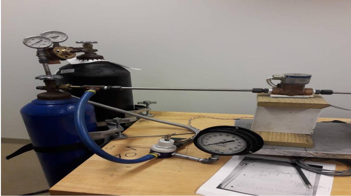
Figure 2.3 Gas launch assembly of in-house SHPB apparatus
