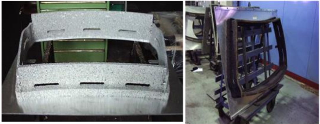
Figure 1.9 Vacuum lifting tool made of Al-foam
