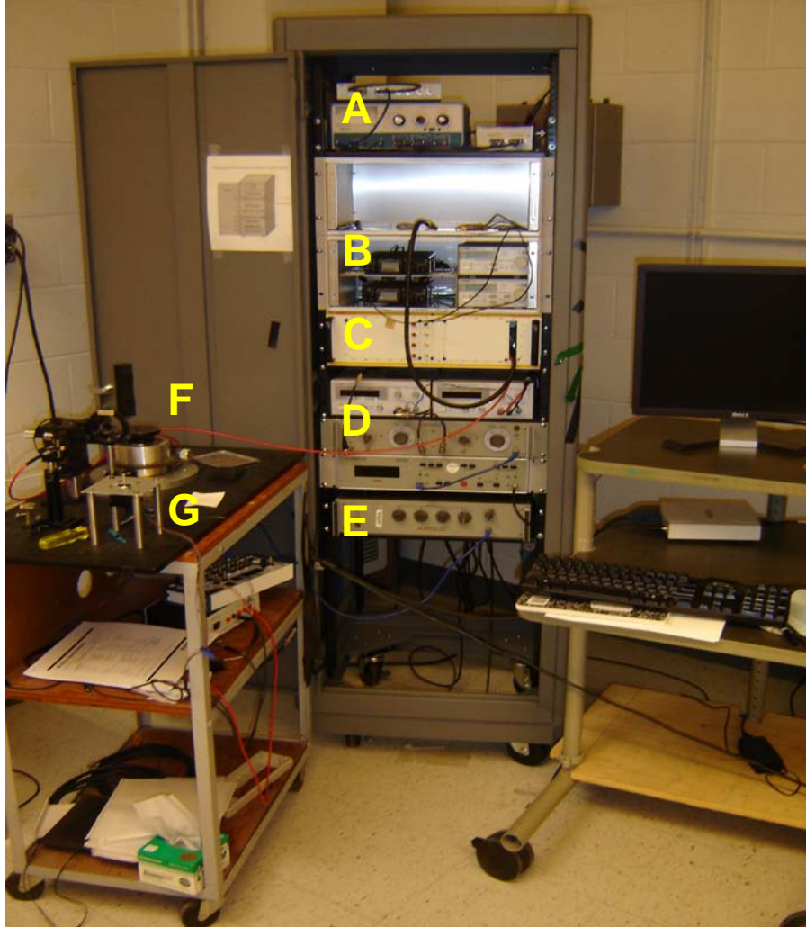
Figure 2.14: Picture of FMT system. A) Reference oscillator, B) Transmitter and Receiver, C) Laser diode mount and PMT (optical components), D) Voltage controller and gain controller for PMT, E) Phasemeter and bandpass filter, F) Fiber optics, and G) Stepper motor and stage.
