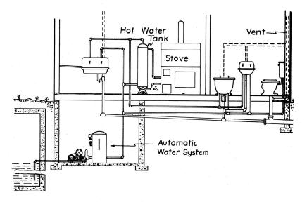
Fig. 3.—A pressure water system makes it possible to supply running hot and cold water to both the kitchen and the bathroom.
