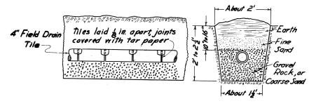
Fig. 8.—Where the soil is very tight, the disposal tile should be laid in a gravel-filled trench.
