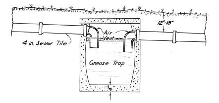
Fig. 10.—If the waste water from the sink contains very much grease, a grease trap should be installed in the drain between the sink and the septic tank.
