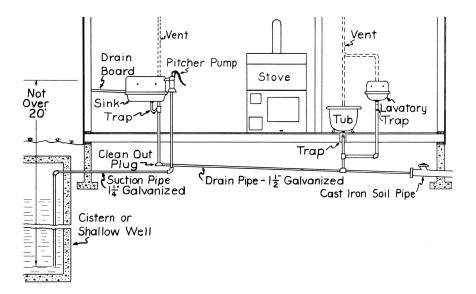
Fig. 2.—A bath tub and lavatory may be installed and connected to the sink drain.
