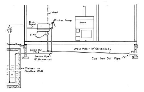
Fig. 1.—A pump, sink, and drain is a practical, simple system which eliminates the drudgery of carrying water into the house, and solves the problem of disposing of much of the kitchen waste.
