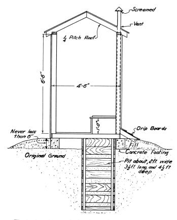
Fig. 4.—A sanitary earth pit privy provides for safe disposal of body wastes where a sewage system is not available.
