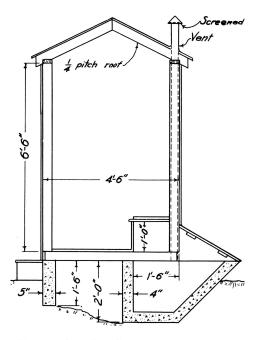
Fig. 5.—Where the soil is very open or where an earth pit privy would endanger the water supply, a water-tight concrete vault privy is recommended.
