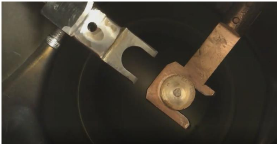
Figure 17. Top-down view of the sample puck transfer between the PEMLD transfer arm fork (left) and evaporation/load-lock/XPS transfer arm fork (right).
