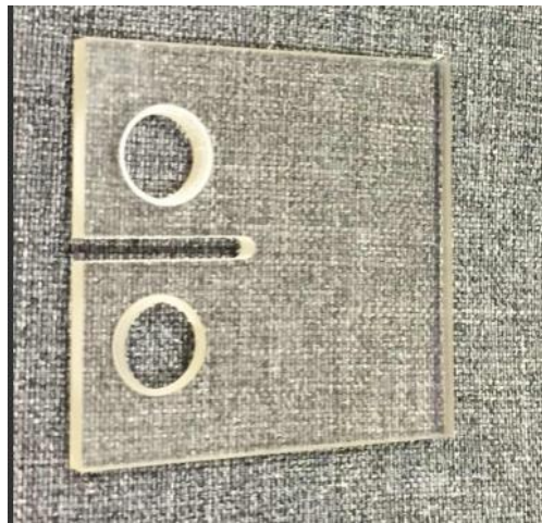
Figure 4.2. CT specimen dimensions and actual test specimen
