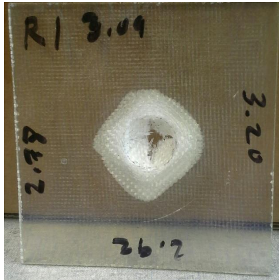
Figure 5.4 Post impact drop weight test specimen
