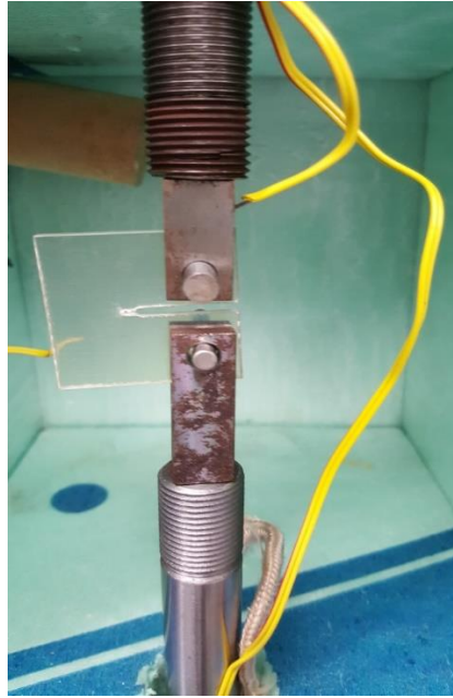
Figure 4.4. Ongoing fatigue crack growth test specimen
