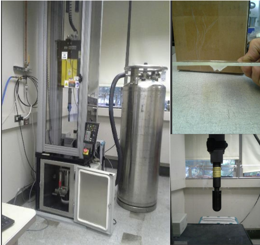
Figure 5.3 Experimental setup of puncture resistance test
