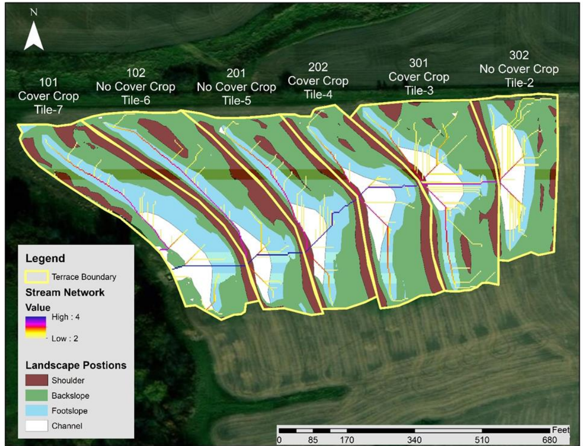
Figure 3.1. Design of the six parallel terraces constructed in 2016. Plots 101, 202, and 301 received a cover crop treatment. Plots 102, 201, and 302 are non-treated controls. Landscape positions are delineated within each terrace.
