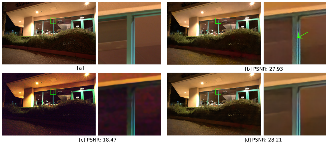
Figure 6: (a) Ground truth image (b) Output from SID. Noise is still present in few parts of the image (c) Output from BM3D. Denoised image is darker than the ground truth. (d) Denoised output from our network
