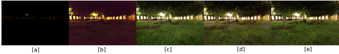
Figure 8: (a) Input dark image form Sony 300x subset (b) 300x amplification of dark image (c) Ground truth image with exposure time of 10 seconds (d) U-Net output with unnecessary color spread at the ground. (e) Output from our network with close approximation to ground truth image.
