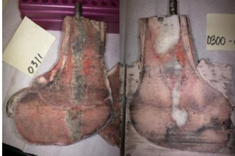
Figure 2.22. Longitudinally cut femurs displaying differences in cement filling between silorane (left) and Simplex™ P (right).
