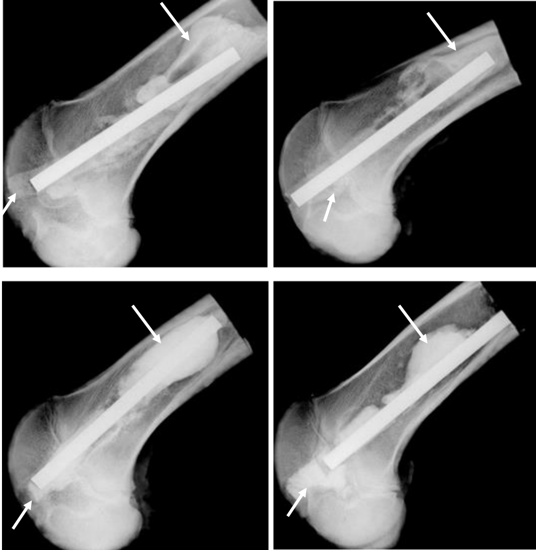
Figure 2.20. X-rays of Simplex™ P (top) and silorane (bottom) pig femurs. The arrows indicate cement location.
