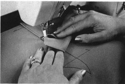
Place trimmed raw edge along pocket line on outside of the garment, extending pocket seam allowance past size line to the other over the line of stitching that formed the welt. Lift pocket as you sew to check placement of raw edge against pocket line.
