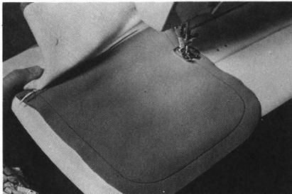
Fold upper section of the pocket down. Sew around the pocket to complete it.
