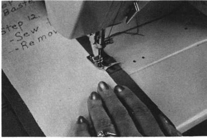
With garment right side out, turn back the garment to reveal the triangles and ends of pocket pieces. Stitch triangles to ends of pocket. Sew back and forth several times.
