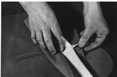
Turn pocket to the inside. Pull ends of pocket to square the corners. *Do not pull on triangles.* The folded edges of the welt should meet in the center.
