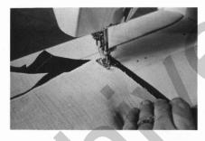
Match the front and back shoulder seams, place the back seam next to the feed dog, and stitch.
