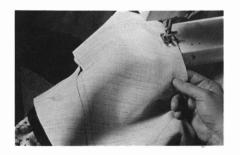
If the machine has a free arm place the sleeve next to the feed dog when stitching. Keep the layers moving smoothly and even by placing the left hand between the jacket and the sleeve. The sleeve should be smoothed by the hand as it moves under the pressure foot.
