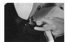
Match the notches, pin the sleeve into the jacket and machine stitch.
