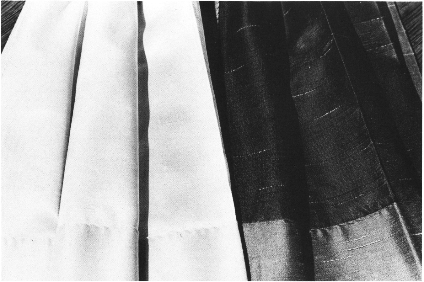
Color of the exposed drapery back affects heat control. Light backs reflect the sunlight; dark backs absorb sunlight.
