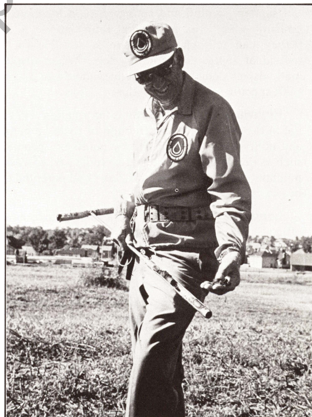
Soil Scientist Les Tobin uses a hand probe to examine each soil type to a depth of 5 feet.
