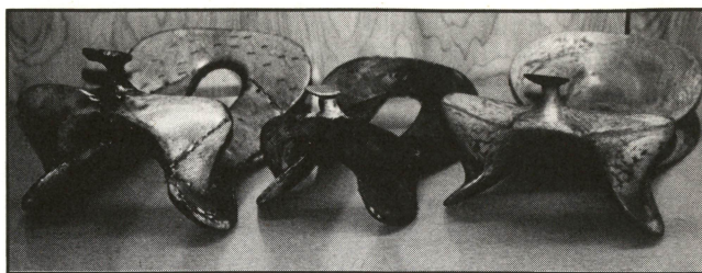
Warp-free saddle forms are made of extruded plastic. Note differences in width.
