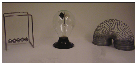
Figure 1. Some of the household objects or toys that can be used in minilabs: a five-ball pendulum, a radiometer and a slinky spring.
