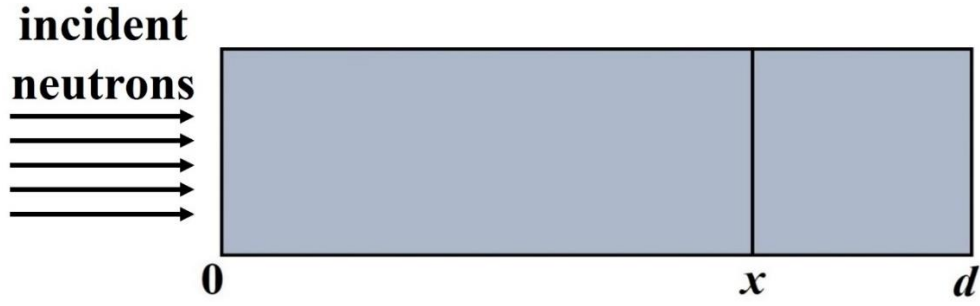
Figure 4. Representation of a detector of thickness d ; x represents a point in the detector at which the incident neutrons are absorbed.
