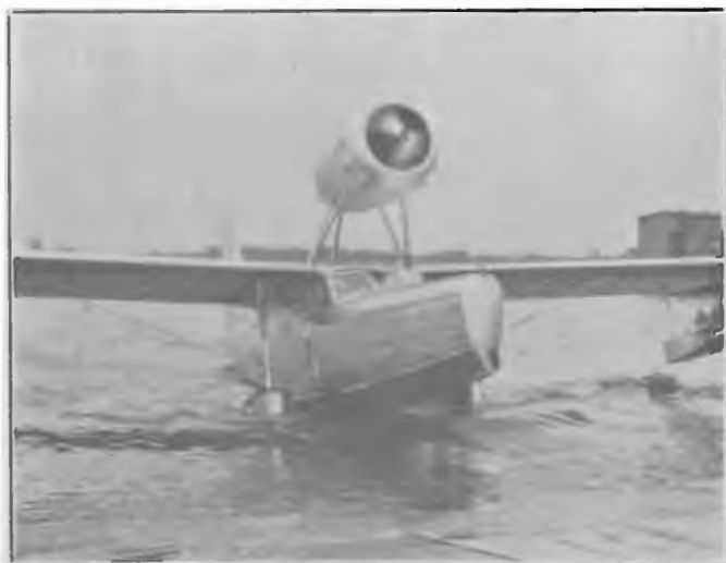
Fig. 1. The Sea Bird. A welded Stainless steel Amphibian fully equipped but weighing only 2,285 lbs.
