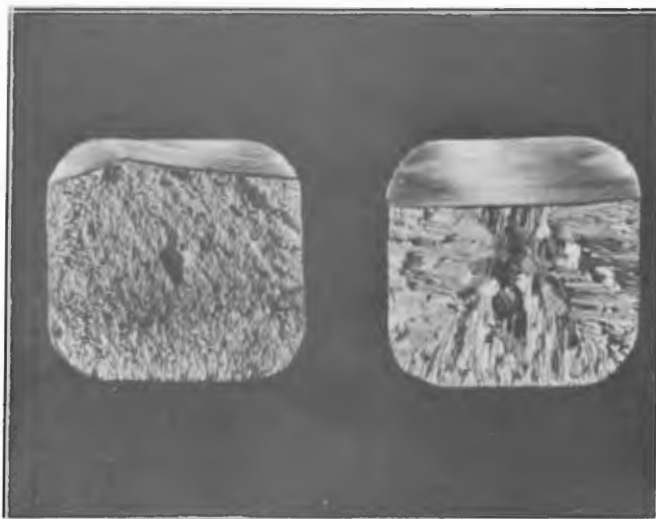
Fig. 2. Specimens showing effect of nitrogen addition on grain size of 20 per cent chromium steel. Left, with Nitrogen. Right, without Nitrogen.
