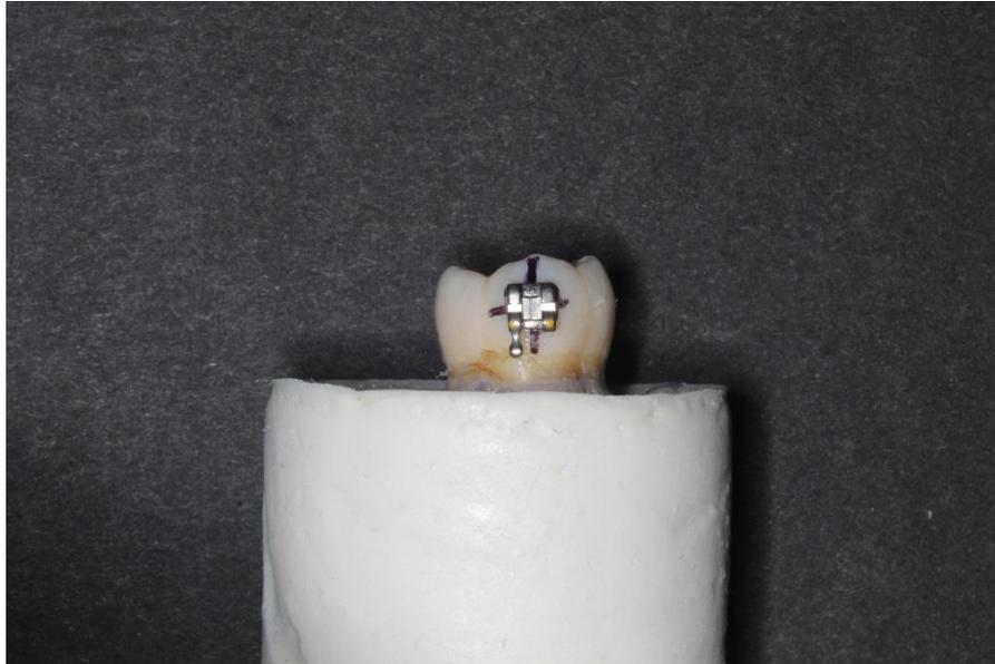
Figure 2. Bracket bonded to mesial buccal of a maxillary third molar.
