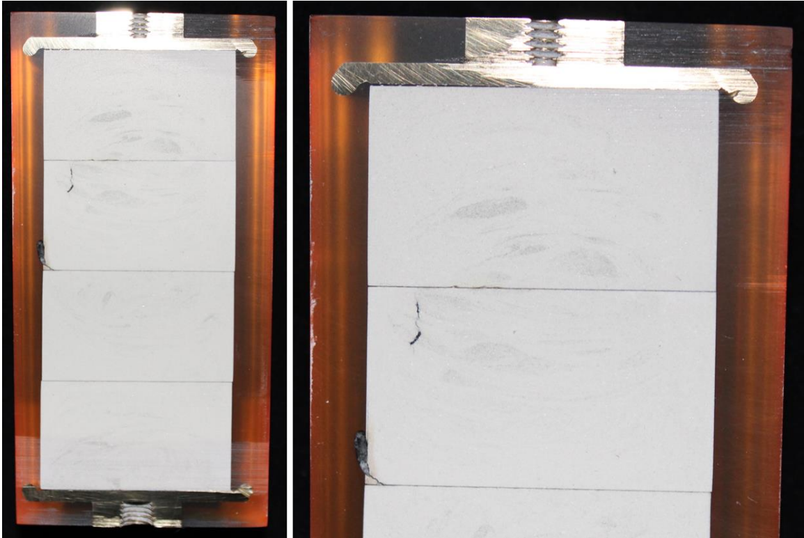
Figure 7.27: After dissection, the breakdown channel through one MU100B substrate is partially visible. The breakdown began within the MU100B material, propagated out, into the encapsulant, then back into the MU100B material.
