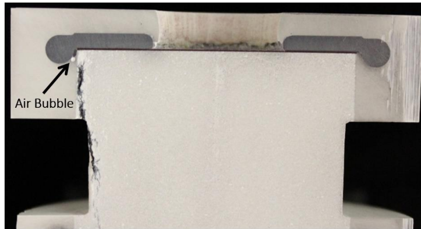
Figure 6.8: Physical shortcomings of the second iteration field shaping electrode trapped air bubbles under the corona ring and allowed for conductive adhesive overflow, resulting in no mitigation of edge breakdowns.
