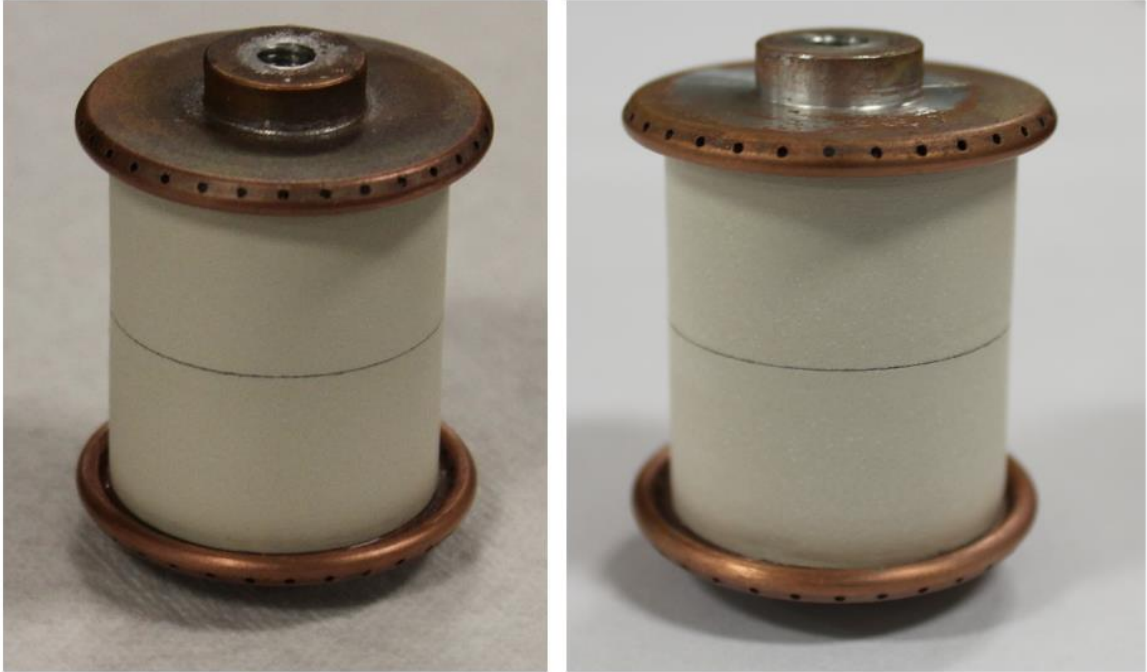
Figure 7.10: The 3.4 cm diameter stacked capacitor that was tested for initial lifetime evaluation at 250 kV. The tests have been carried out on the capacitor as shown, unpotted, just submerged in oil, where it has withstood 10,000 shots from the 250 kV test stand. The image at the left is the capacitor before any testing. The image at the right is the same capacitor after surviving 10,000 shots. No signs of degradation have been observed.
