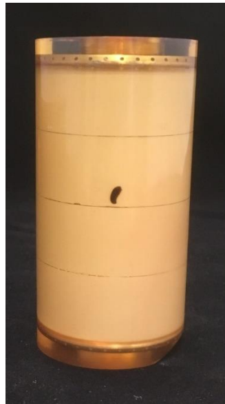
Figure 7.26: Sub-module #11 after failure. The carbon buildup is due to the breakdown tracking out of the MU100B material into the encapsulant.
