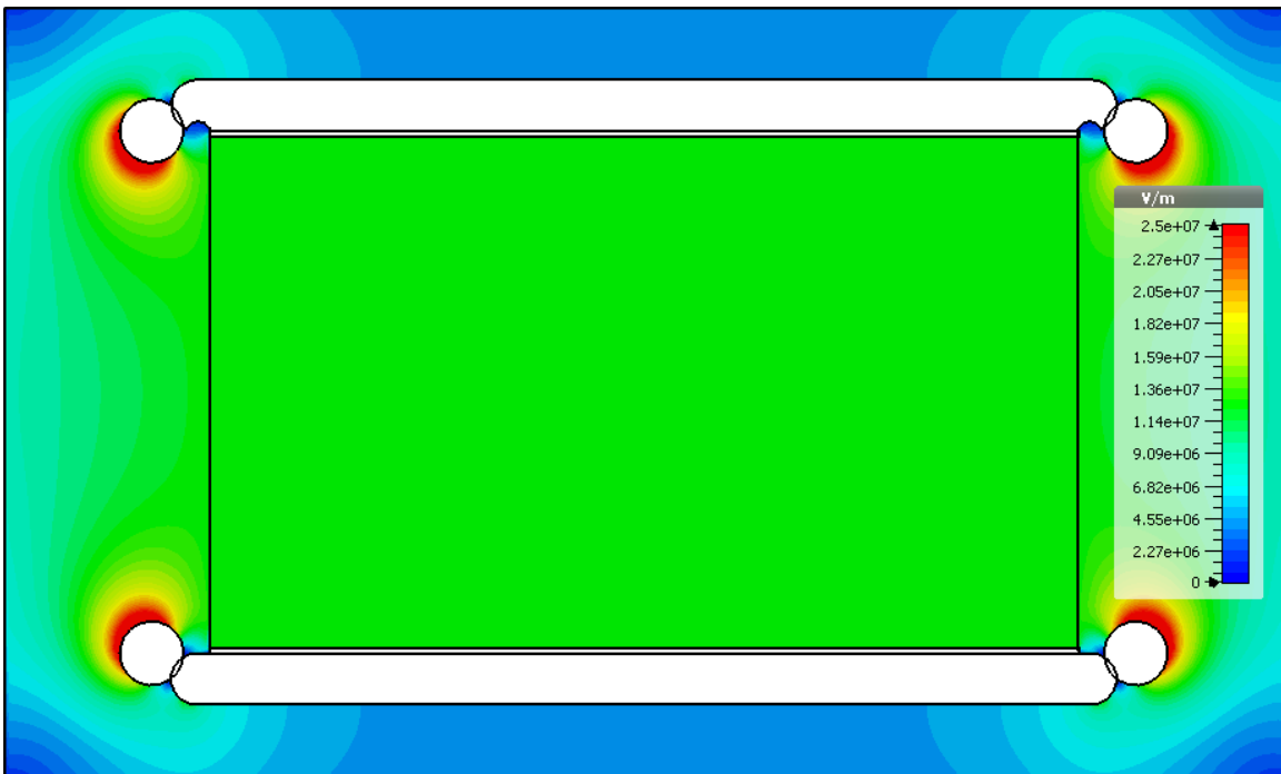
Figure 6.6: Electrostatic model of the second iteration field shaping electrode. The major inner radius of the corona ring was expanded to give 0.1 cm of separation between the field shaper and the MU100B, allowing the fields in the MU100B to be less distorted by geometry changes.
