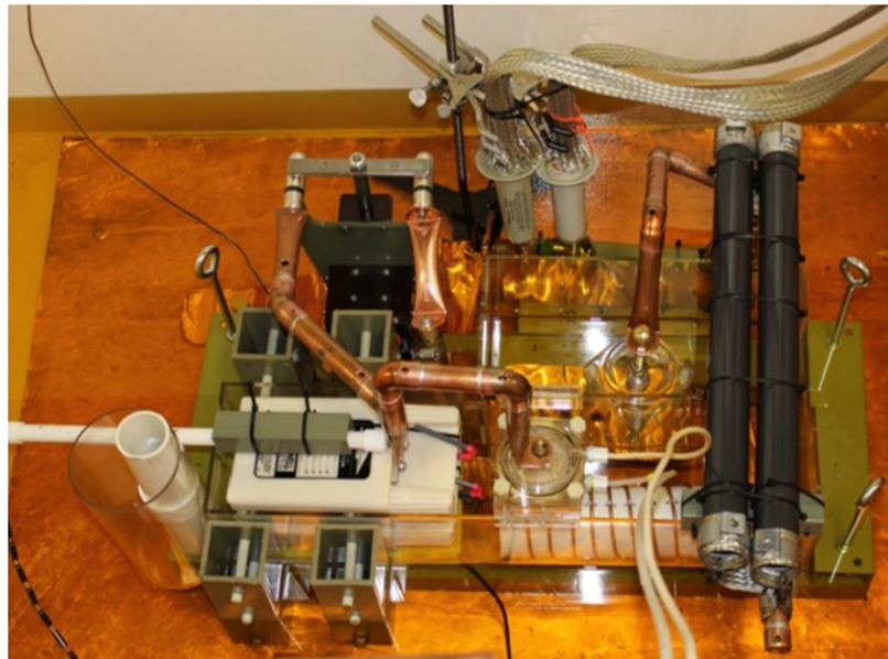
Figure 4.9: Iteration two of the 250 kV Test Stand. Addition of copper pipe conductors and higher power components enabled test stand operation in repetitive mode at a pulse frequency of 1 Hz.
