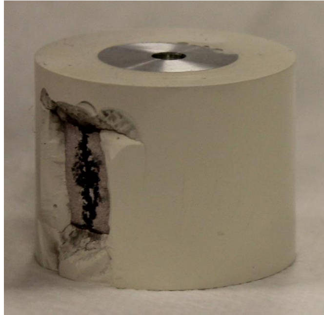
Figure 6.2: A scaled, flat electrode edge breakdown. The high field enhancements at the triple point lead to edge failure at \sim 80 kV/cm average field (400 kV/cm at enhanced points) [2].
