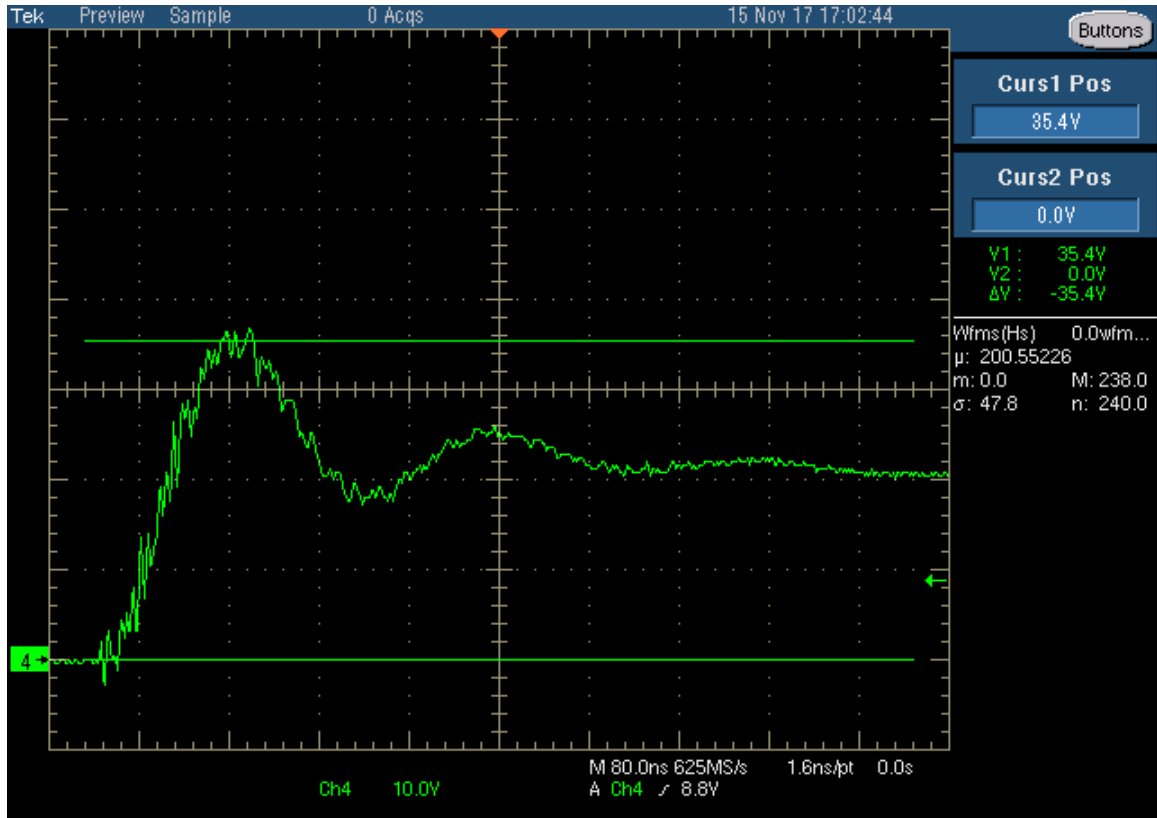
Figure 7.11: The 10,000th shot put on the preliminary stacked 3.4 cm capacitor. The voltage per division of the plot, including voltage divider attenuation, is 72.5 kV per division, giving a peak voltage of 256.7 kV. The time axis is 80 ns per division. Characterization of the test stand showed that voltage is left on the sample for \sim 10 \mu\text{s} .
