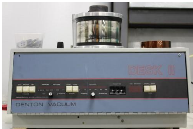
Figure 3.2: Denton Desk II DC sputter coater developed by Denton Vacuum used to deposit conductive silver (Ag) as electrodes onto sample capacitors. Sputter coating allows for some surface penetration of the sample as well as surface deposition resulting in a greater metal-substrate interface [2].
