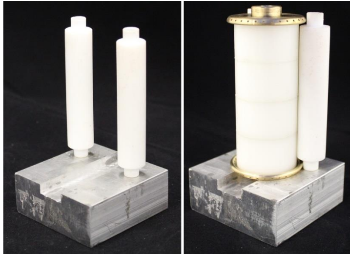
Figure 7.3: Stacking jig used to ensure concentric stacking of 500 kV capacitor elements (left). The jig is shown with a stacked element on right.
