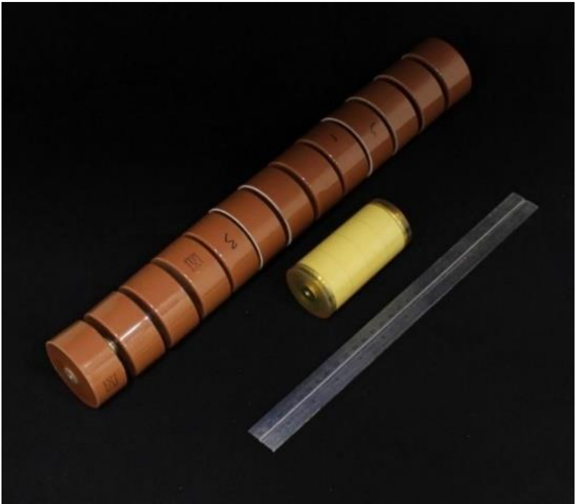
Figure 7.6: An encapsulated 500 kV capacitor prototype (center) is shown next to a 500 kV assembly of TDK door knob capacitors (left) along with a ruler for size reference. The capacitor development effort resulted in 500 kV capacitors that fit in the palm of the hand.
