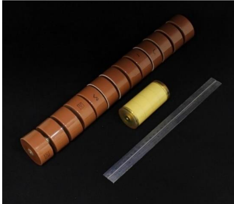
Figure 8.1: A 500 kV MU100B sub-module shown side by side with a 500 kV stack of commercially available ceramic capacitors and a standard ruler for size reference.
