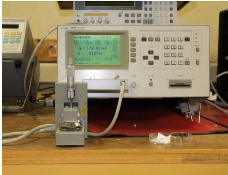
Figure 4.1: Agilent 4285A Precision LCR Meter used to gather low voltage dielectric measurements over a range of frequencies, 75 kHz up to 30 MHz. Per the ringing nature of the ultimate application, most concern was put on frequencies between 5 and 15 MHz [1].
