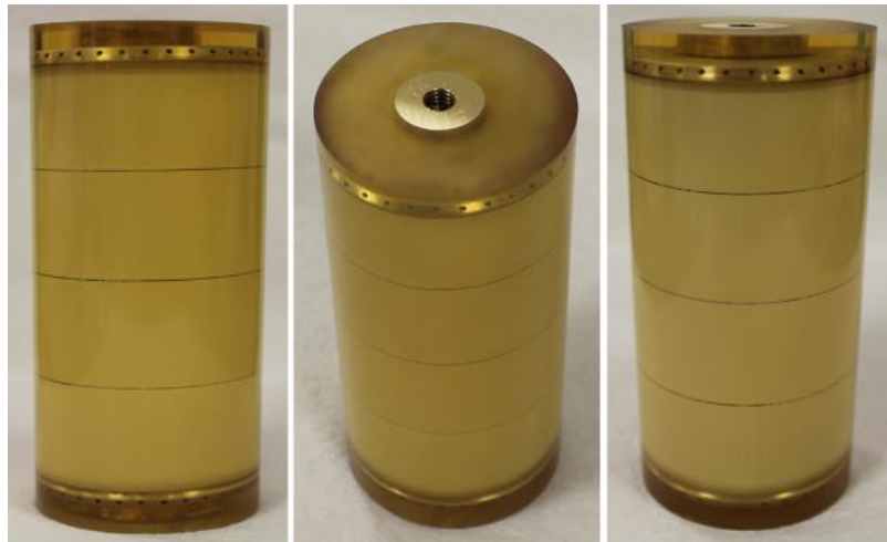
Figure 7.13: Photograph of various sub-modules which comprise the 500 kV capacitors. The sub-module capacitors are 9.5 cm in length with a diameter of 4.5 cm.
