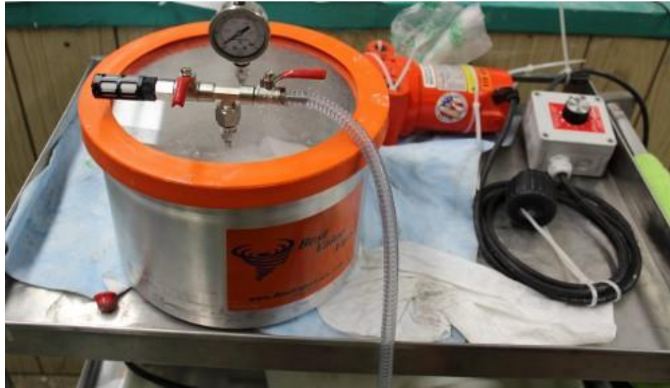
Figure 3.4: Vacuum chamber used when encapsulating ultra-high voltage capacitors. Out gassing is used to reduce the prevalence of voids in potting compound. Vacuum is reached with a roughing pump capable of reaching 29 in. Hg.
