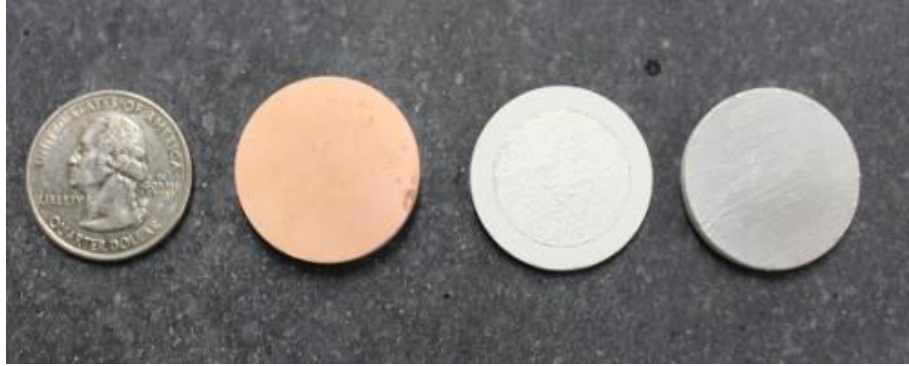
Figure 3.1: Comparison of samples from different electrode generations. From left to right: a USA quarter for size comparison, generation 4 sample with full radius electroplated copper electrode, generation 2 sample with inset silver loaded epoxy electrode, and generation 3 sample with full radius painted silver electrode [1].
