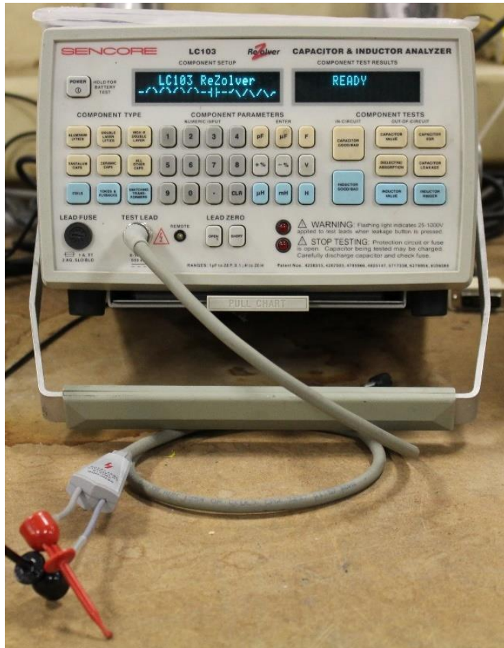
Figure 4.3: Sencore LC 103 Capacitor and Inductor Analyzer. The primary characterization function of this instrument is to take a high voltage leakage resistance measurement. If leakage resistance measures too low, samples are discarded [4].
