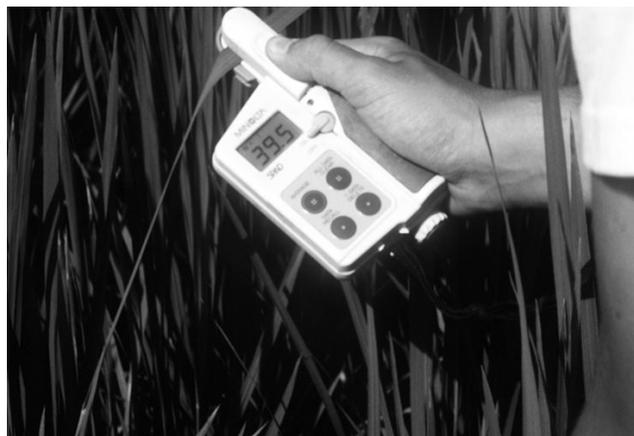
Figure 1. Measuring green pigment in rice plants with a Minolta SPAD chlorophyll meter.
