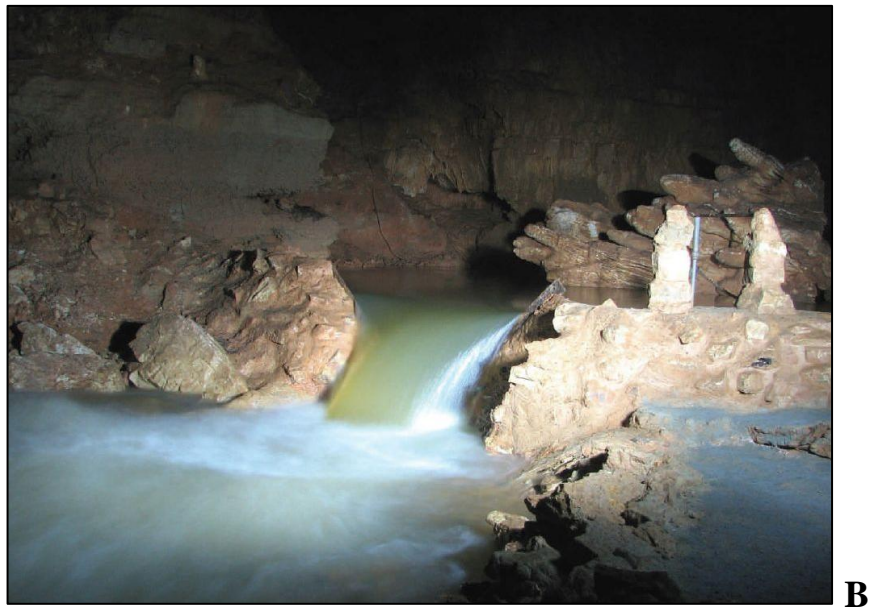
Figure 3.1. (A) The TCC gauging station showing staff gauge and stilling well at the weir, directly upstream from study reach. A pressure transducer and data logger was used to record water height and temperature. (B) High flow event at the V-notch weir in TCC used to correlate stage with discharge. The discharge during the time the picture was taken was approximately 2.5 \text{ m}^3 \text{ s}^{-1} .
