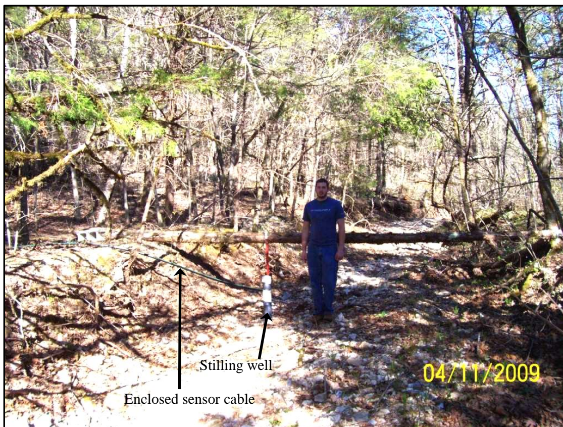
Figure 3.2. View of the BCH gauging station located approximately 10 m from the upstream end of the study reach, looking downstream to the east. A Global Water Instrumentation, Inc. WL16 pressure transducer was used to record water height and temperature during flow events. The sensor sits ~ 10 cm below the surface of the stream bed within the depicted 15 cm diameter PVC pipe (stilling well) installed in the thalweg of the channel. The stilling well is secured in place by a fence post attached to a tree trunk laid perpendicular across the channel. The average bank height here is approximately 0.71 m.
