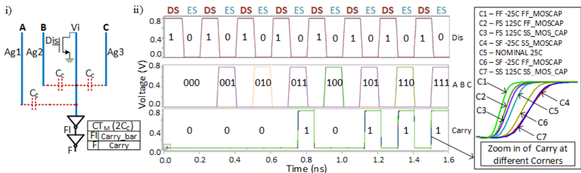
Figure.10.5. i) Crosstalk CARRY Circuit Schematic, ii) Extracted Circuit Simulations at different Corners
