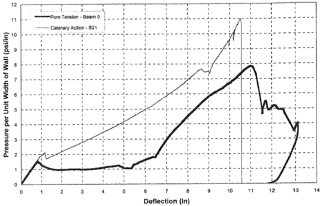
Figure A2.3: Pure Tension Action verses Catenary Action
