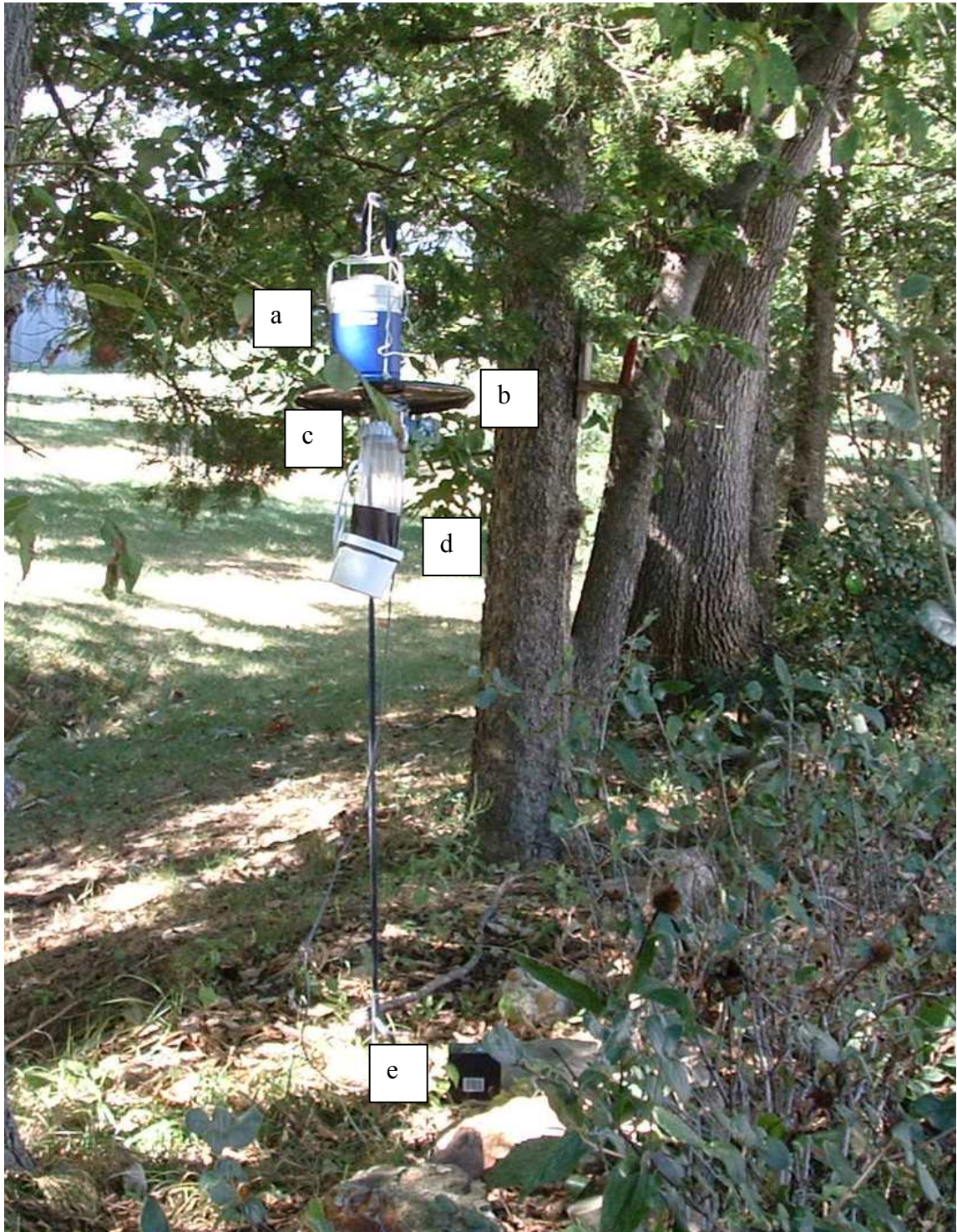
FIGURE 2 — CDC mini-light trap used for mosquito collection in this study.
