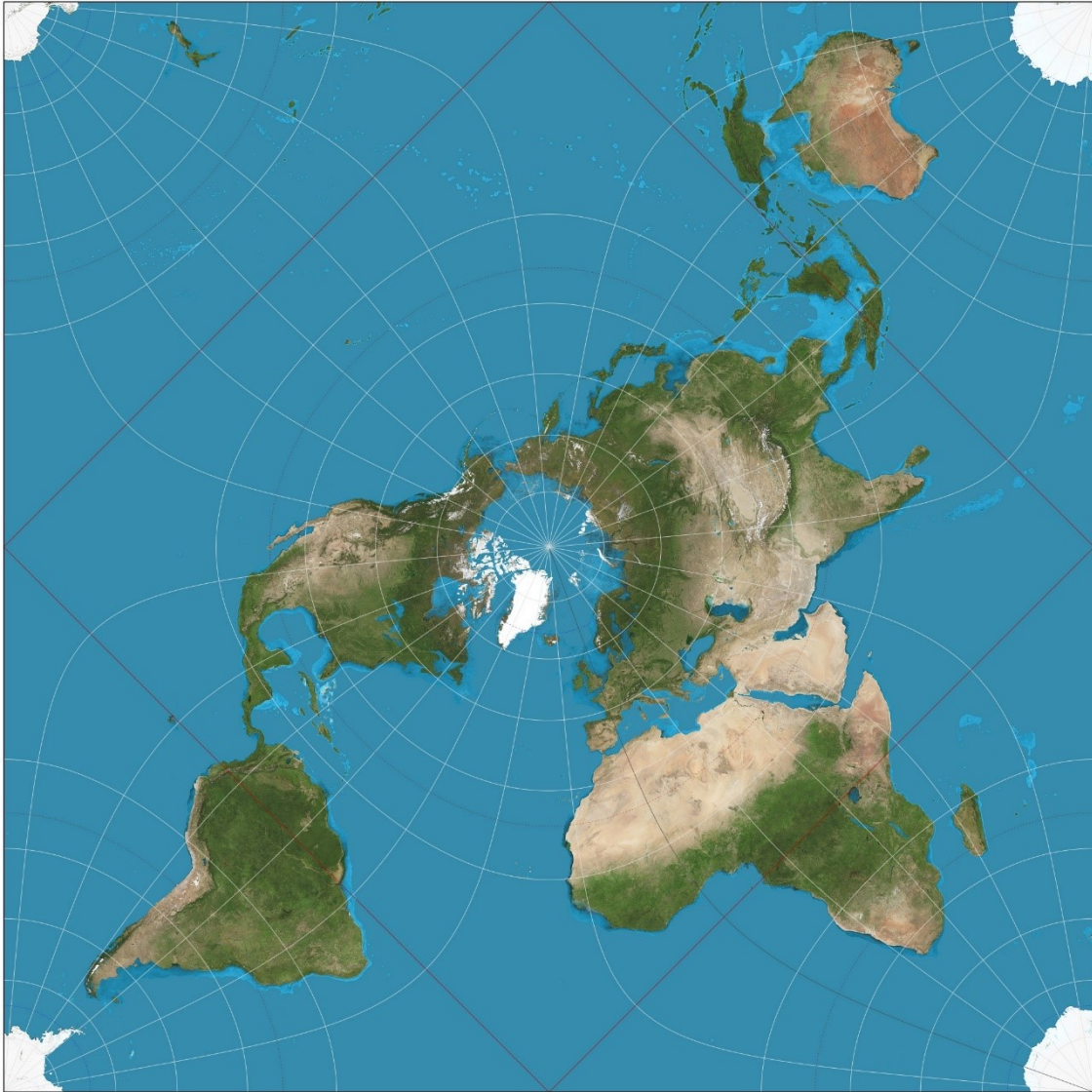
Figure 2.3. Peirce's quincuncial projection. From "Peirce quincuncial projection," by D. R. Strebe, 2012, CC BY-SA 3.0.
