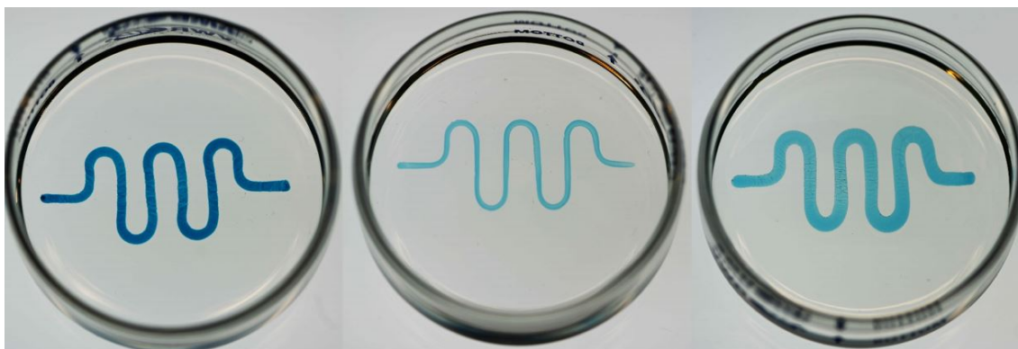
Figure 5: Printing of 2D planar designs (meandering channel) within an oil phase using aqueous solution of different types of surfactants. From left to right, the aqueous solutions contain SDS, F68, and CTAB.
