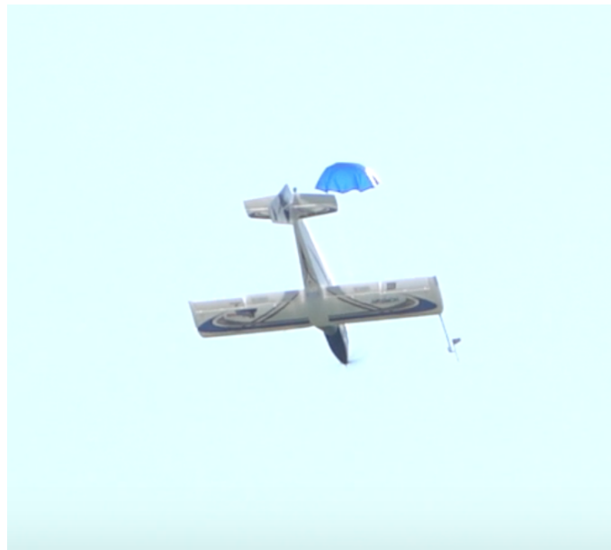
Figure 37: Timber UAV nosedive trajectory during the wing bay payload failure.
