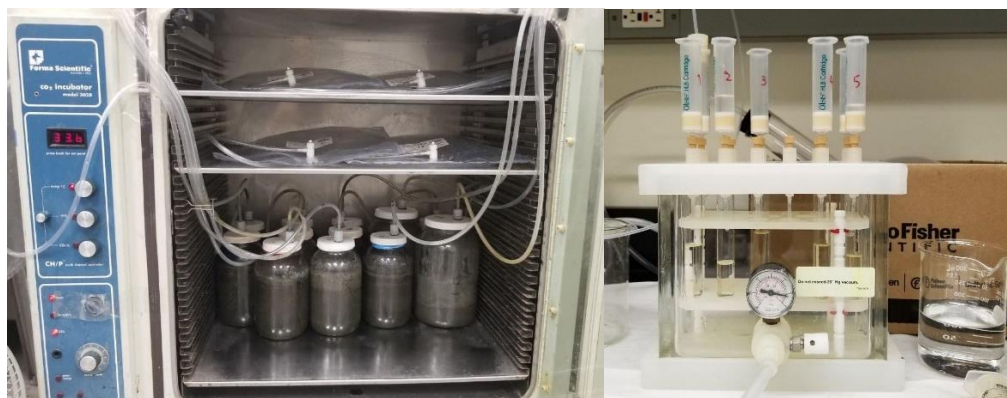
Figure 1. Left) The scheme of the reactors, tubes transferring biogas, and the incubator, Right) Solid-phase extraction step.
