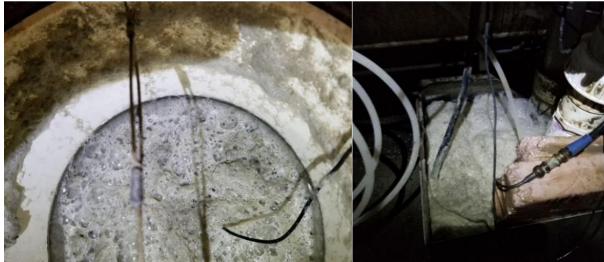
Figure 13. Foaming issue, left foaming happens in the acid tank; right foaming happens in the reservoir.
