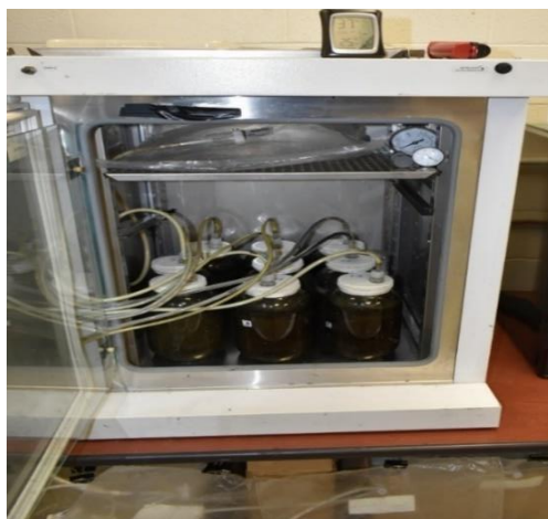
Figure 1. The scheme of the reactors, tubes transferring biogas and the incubator.
