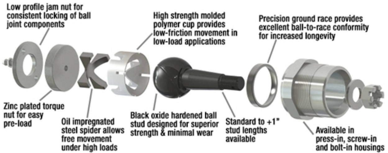
Figure 27 - Exploded View of QAI Ball Joint [20]
