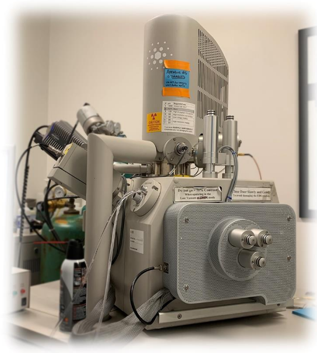
Figure 3-9: FEI Quanta 600 FEG Environmental SEM
