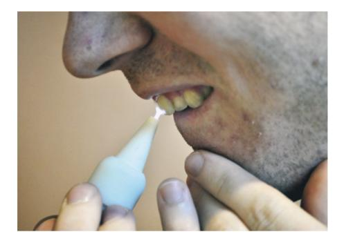
Andrew Ritts demonstrates the plasma dental brush, which in less than 30 seconds can disinfect and clean cavity holes before fillings are placed. *Photo courtesy of the College of Engineering.*
