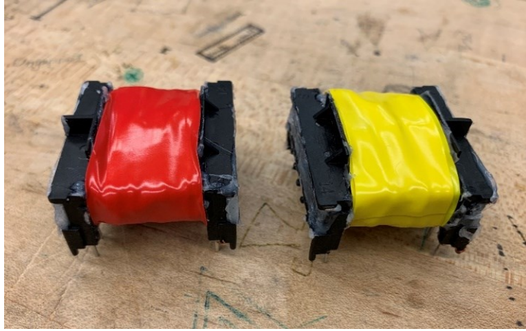
Fig. 50: Custom isolation transformers for the isolated gate driver
