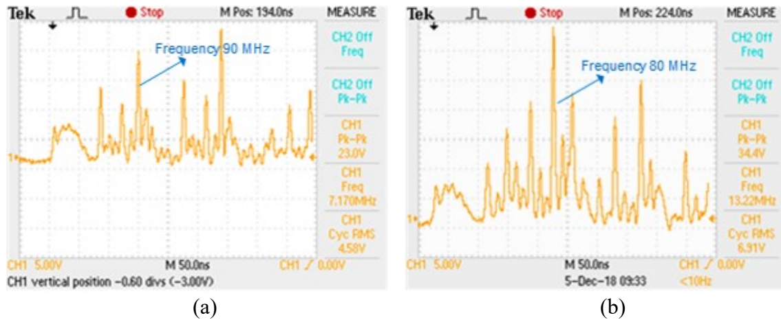
Fig. 24: Output from (a) 600 V rated Schottky diode based NLTL ( V_{DD} = 10 V) (b) 1200 V rated Schottky diode based NLTL ( V_{DD} = 10 V)
