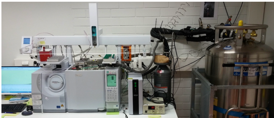
Figure 1. 4. A comprehensive two-dimensional gas chromatography-mass spectrometer used for breath analysis. Adopted from ref 6.
