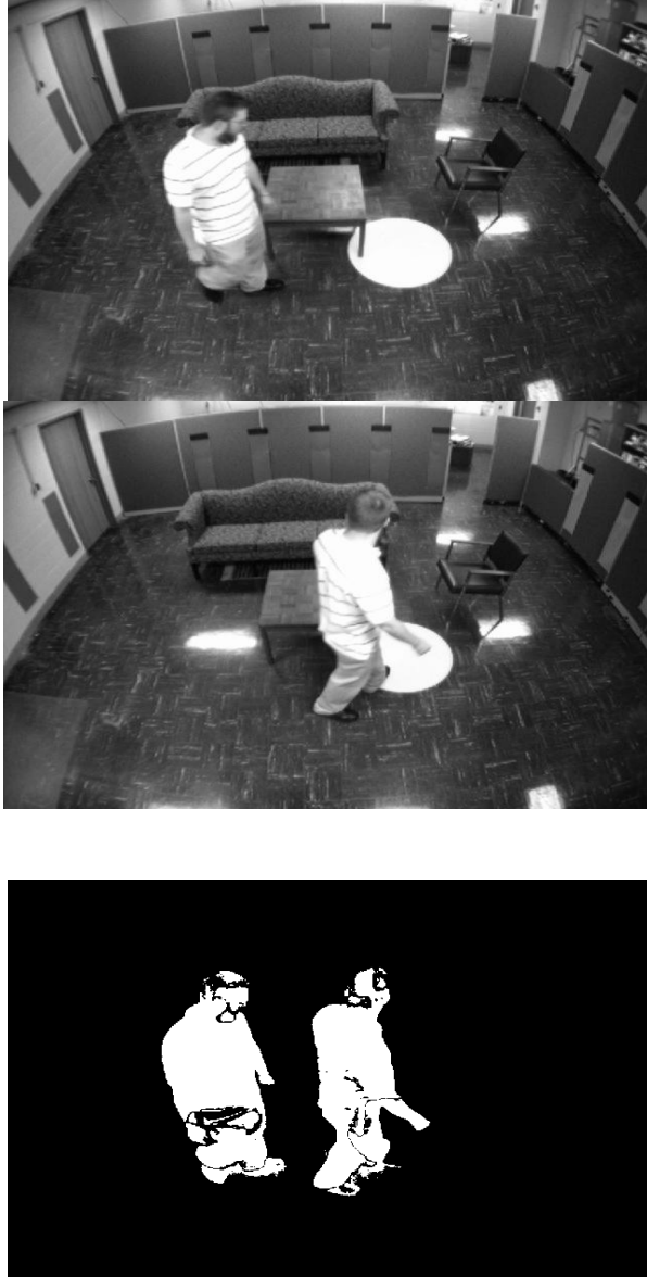
Figure 2.1: An example of the double foreground phenomenon produced by temporal differencing. The person is in the current frame as well as the previous. His locations are then classified as change between the frames.
