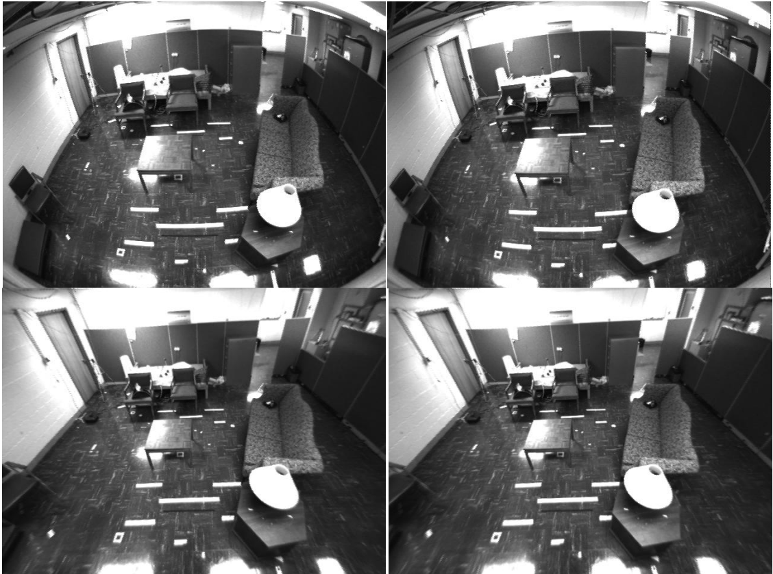
Figure 3.1: Left and right images in a stereo pair is shown in the top row. The bottom images show the epipolar rectified images.
