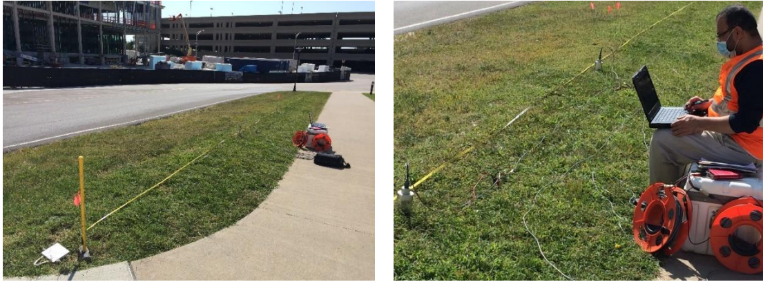
Figure 3.20 Test setup and equipment used for SASW and HWAW methods for Site 1.
