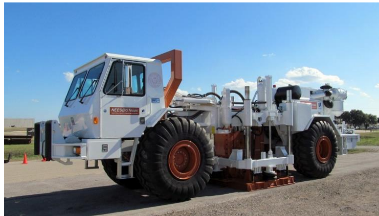
Figure 3.22 Low-frequency NEES vibrator (from: http://nees.utexas.edu/Equipment-Liquidator.shtml ).
