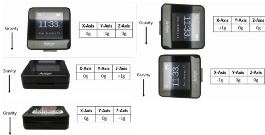
Figure 2.2-1 ActiGraph GT9X Link device orientation with respect to the X-axis, Y-axis, and Z-axis.
