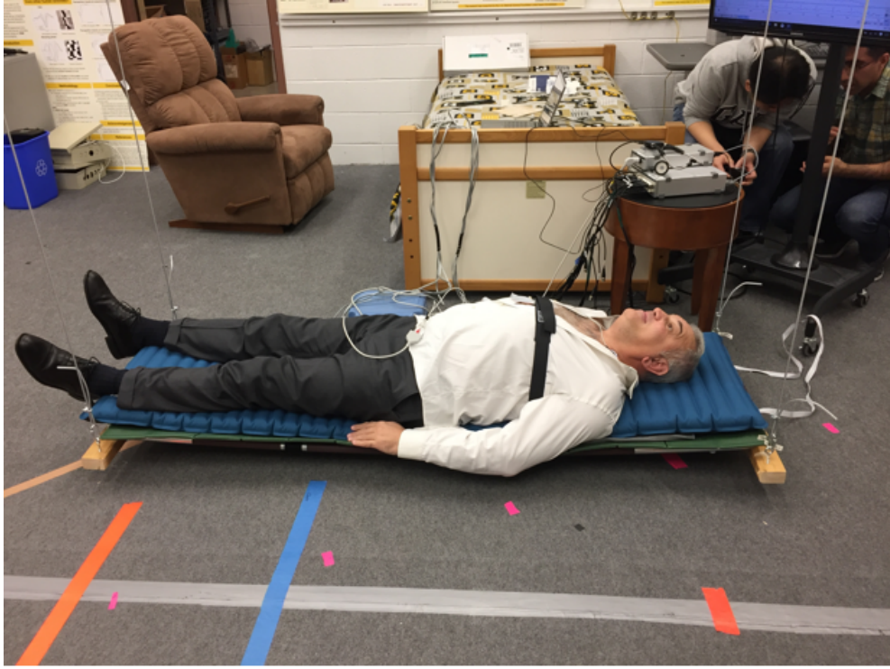
Figure 2.5: Replica of the suspended ballistocardiography bed originally designed by Burger, et al. [8], utilized in the present work.
