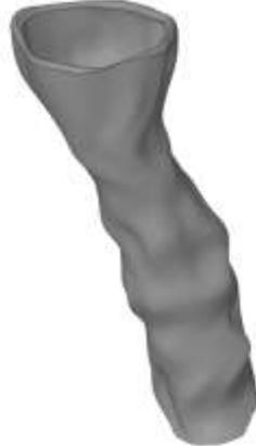
The refined 3D model generated in the CAD software was imported as a parasolid into the CFD compatible CAD design software. Part volume was automatically assigned as the fluid body when imported into the software. The inlet and walls were assigned by named selections to define the geometric boundary conditions. The inlet was defined as the start of the cross section of the ONSAS and the ONSAS outer diameter was
